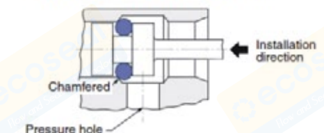
Fig. 1.5.2 Chamfer of pressure-hole edges
