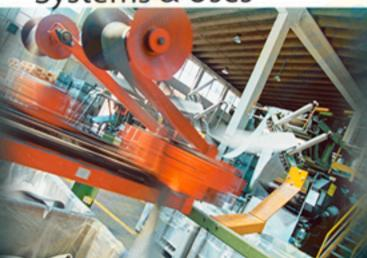
Black compounds are produced with a 200-litre Banbury mixer. Coloured compounds are produced with a 130-litre Banbury mixer. All systems are fully PLC-controlled and are equipped with automatic dispensers for Carbon Black, non-black fillers and plastifying additives; the other chemicals are added separately by a specially designed automatic feeding system.
