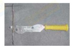
"Sure-Pull" Extraction Hook Puller showing a flexible extraction hook in place.
