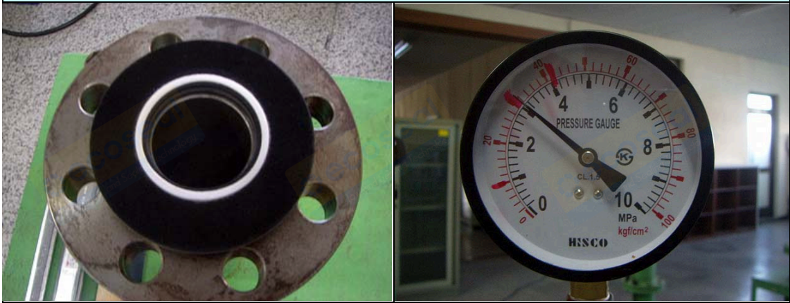
Nitrogen Pressure (31kg/cm 2 ) : No leakage
