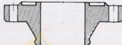
Large Tongue and Groove Joint
