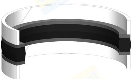
K503 is a five piece double acting compact seal which consists of one elastomeric nitrile rubber sealing element, two polyester elastomer back-up rings on both sides to prevent extrusion into the sealing gap and two special profiled guide rings produced from thermoplastic to absorb transverse forces.
