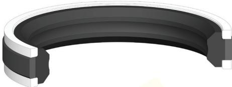
K48 is a four piece double acting heavy duty piston seal which consists of one TPE profile ring, one elastomeric nitrile rubber to pre load sealing element and two thermoplastic back-up rings.
