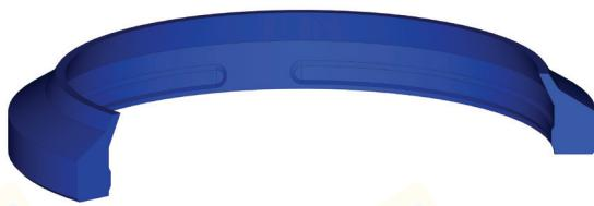
K93 is a single acting wiper ensuring that foreign particles are not introduced into the hydraulic system.
