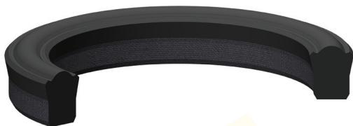
K39 is a single acting rod seal which consists of reinforced cotton fabric and nitrile rubber vulcanized together forming an integral sealing element.
