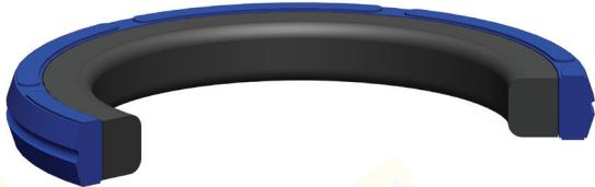
K49 is a two piece double acting sealing set which consists of a special design polyurethane seal ring and a NBR elastomer ring as energizer.
