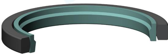
K704 is a two piece single acting rod seal which consists of one special mixture PTFE profile ring and a NBR elastomer ring as energizing element.
