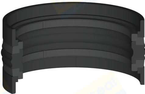
K518 is a five piece double acting compact seal which consists of one elastomeric nitrile rubber sealing element, two polyester elastomer back-up rings on both sides to prevent extrusion into the sealing gap and two special profiled guide rings produced from thermoplastic to absorb transverse forces.
