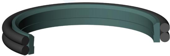
K705 is a three piece single acting wiper which consists of one special mixture PTFE profile ring and two o-rings as energizers. K705 ensures that foreign particles are not introduced into the hydraulic systems, avoiding wear and damage to all the internal components including seals.
