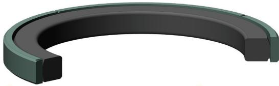
K755 is a two piece double acting piston seal which consists of one energizing elastomer ring and special mixture thermoplastic ring.
